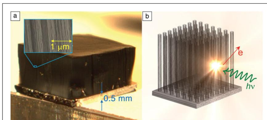
**Figure 1.** (a) Photograph of a millimeters-tall multiwalled carbon nanotube (CNT) forest, with the scanning electron micrograph (inset) revealing its nanostructure. Reprinted with permission from Reference 42. © 2015 American Chemical Society. (b) Schematic (not to scale) of a heat trap experiment, where incident light locally heats the CNT forest, leading to localized incandescence and thermionic emission. Note:  $h$ , Planck's constant;  $\nu$ , frequency.
