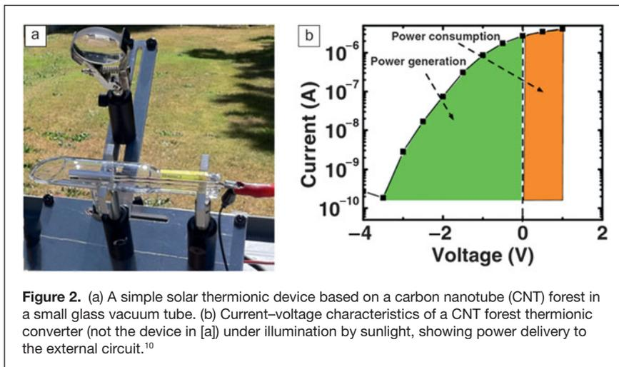
**Figure 2.** (a) A simple solar thermionic device based on a carbon nanotube (CNT) forest in a small glass vacuum tube. (b) Current–voltage characteristics of a CNT forest thermionic converter (not the device in [a]) under illumination by sunlight, showing power delivery to the external circuit.<sup>10</sup>
