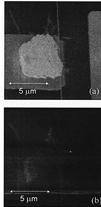
FIG. 5. Imaging and stimulated field-emission at a low primary beam acceleration voltage of 500 V. (a) Zero bias—normal SEM image; (b) applied bias is  $-30$  V. Note that stimulated emission is hard to obtain at this low value of primary beam acceleration voltage, and only one of the nanotubes exhibits the phenomenon.
