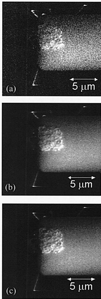
FIG. 4. Stimulated field-emission under various video sample averaging methods: (a) point by point; (b) line by line; (c) frame by frame. Applied bias:  $-49$  V. Number of samples averaged: 32. (Primary beam acceleration voltage: 3 kV.) Note that in line or frame modes, the streaks emanating from nanotube tips are longer than in the point mode.
