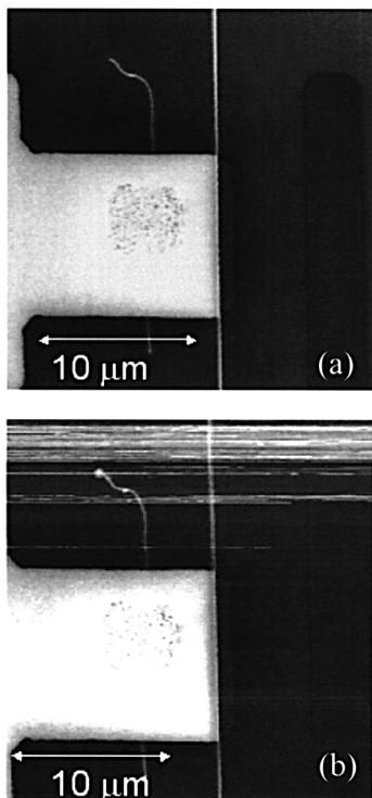
FIG. 2. (a) Voltage contrast. A voltage of  $-24$  V is applied to the nanotubes with respect to ground (the gate electrode on the right). (b) Applied voltage is  $25$  V. Stimulated field-emission can be seen as a bright spot on the nanotube tip. The bias voltage is right at the spontaneous emission threshold, and some traces of spontaneous emission can be seen as white stripes on the top portion of the image. (Primary beam acceleration voltage:  $5$  kV.)
